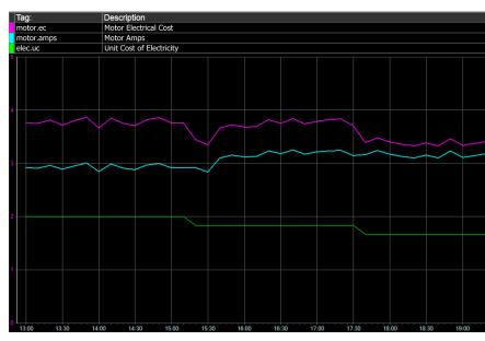
Combining ERP electricity cost data (green) with the amps produced by the motor (blue) to calculate the electrical cost of operating the motor (pink).
